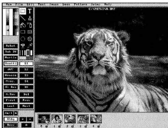
Figure 4.10. An example of the Main Menu Screen for John Langner's Pasokon TV Lite software. An image, whether received off the air or recovered from disk, occupies most of the screen. The extreme upper left of the screen contains a graphic tuning indicator. To the right of the indicator is a box of graphics tools that function much like a basic paint program, permitting you to add text to any image, add graphical effects, and perform many other specialized functions. Below the tuning indicator, arrayed down the left side of the screen is a series of boxes for the major SSTV mode “families.”
