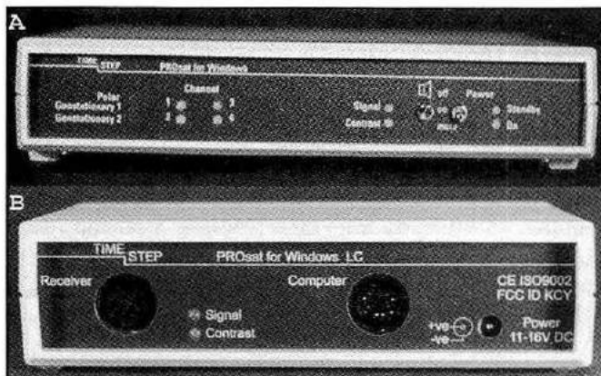
Figure 7.2. An example of two external interface units from TimeStep, Ltd. [A] is their top-end PROsat for Windows while [B] is the less-elaborate PROsat for Windows LC . Both units interface to the station computer, using a high-speed serial port.
