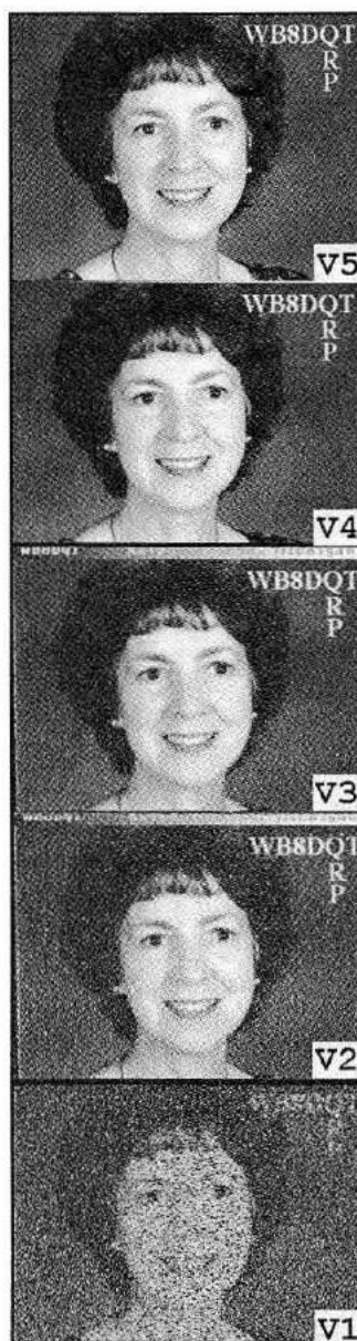
Figure 5.11. The video (V) component of the SSTV RSV signal reporting system attempts to provide a concise but subjective report of the image signal-to-noise ratio. The scale, as shown here, ranges from V5 (an image that is essentially "closed-circuit" with no noise) to V1 (noise dominated, but with some definable image content). V0 is not shown as it would represent a frame dominated by noise with little, if any, image content.
