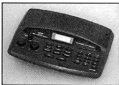
Figure 6.14. The Multifax receiver is based upon a commercial scanning receiver, which has been modified for satellite reception.
