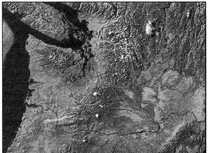
Figure 6.4. The NOAA HRPT multi-spectral imaging format provides a resolution of approximately 1.1 km at the sub-point — the point directly below the spacecraft at any given moment. This is just a small segment of the HRPT channel 1 (visible) data as the spacecraft was passing over the Pacific Northwest. The Columbia River is clearly delineated along the lower edge of the image segment, and the eastern end of Vancouver Island appears in the upper left. Snow cover is clearly visible on the mountains of the Olympic Peninsula and the northern Cascades.
