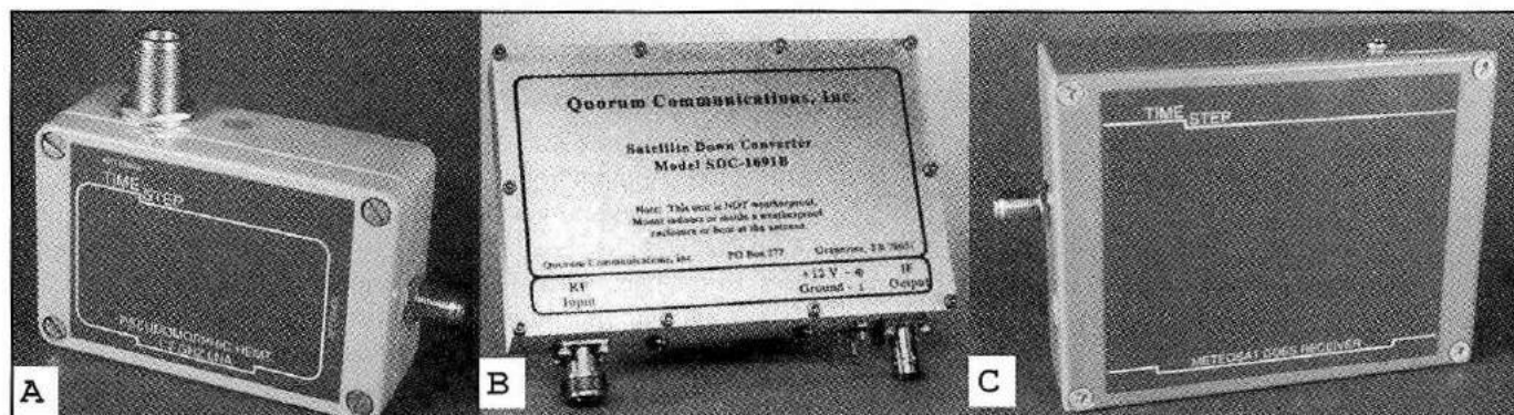
Figure 6.19. GOES/METEOSAT receiving hardware. [A] A remote preamplifier (LNA) mounted at the antenna feed is essential if there is any significant length of transmission line between the feed point and the down-converter/receiver. This TimeStep unit is housed in a weatherproof case, which simplifies installation. [B] A down-converter is used to convert the 1691.0/1694.5 MHz WEFAX signal to the 137-138 MHz range (typically 137.5 MHz) where the polar orbit satellite receiver can be used to demodulate the signal. This Quorum Communications converter features an internal crystal oven that maintains the stability of the local-oscillator frequency despite wide changes in ambient temperature. With a suitable weather-proof housing, this converter can be mounted at the antenna, in which case no preamplifier is required. If such a converter is installed inside with the receiver, a remote preamplifier will be required. [C] This TimeStep unit is unique in that it is a complete WEFAX receiver, incorporating the down-converter and IF receiver components. The output is an audio signal that can be routed directly to the image demodulator/interface.
