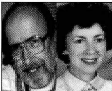
Figure 3.11. An example of two 32-line pictures as transmitted by the NBTV ROMScanner.
