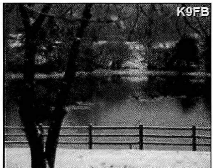
Figure 10.1. An off-the-air example of the new 43-second medium resolution monochrome SSTV format incorporated into the multi-mode MixW software.
