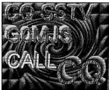
Figure 5.9. Computer sound card clock errors result in a “slant” on received and transmitted images. This picture (320 × 240) was received from GOMMS right after my ChromaPix software was installed on a new computer, resulting in a slight slant to the left, best observed by looking at the right margin. All SSTV software has provisions to correct these clock errors.
