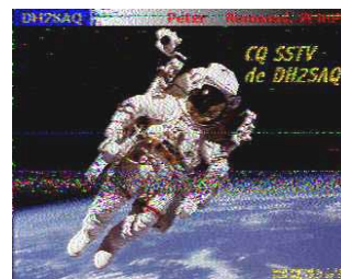
Weak-signal SSTV on 10 meters! This image was copied from DH2SAQ at 6:30 AM my local time. The signal audio was weak and the S meter was reading zero.
