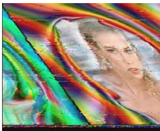
Figure 4—If you see an image like this, you need to adjust your slant (see text).
