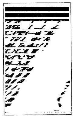
This picture section is leaning to the right, and unwanted line feeds were inserted during reception. The extraneous line feeds were caused by the presence of an unneeded—for the Epson FX-286—printer command; see text.
