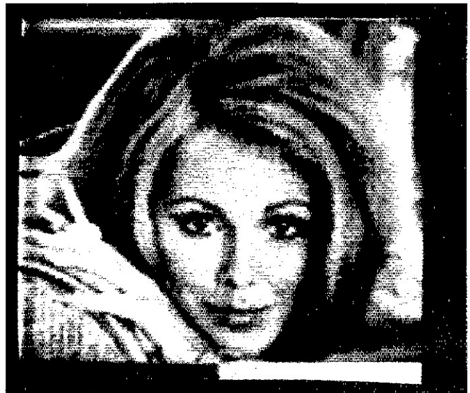
is one means of smoothing out the effects of contouring, as shown here. At the left is a 128 by 128 picture-element slow-scan picture with 16 brightness levels. At the right is the same picture except for the addition of pseudo-random noise.
