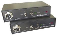
RIGblaster by West Mountain Radio provides all digital modes send and receive in this rugged black sound card radio interface. Includes cables and software for virtually all digital modes. Price is \$129.95 from Universal Radio. (Courtesy: Universal Radio)
