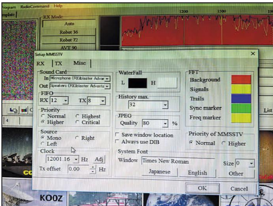
Photo G. The MMSSTV Misc tab is where the sound card being used for SSTV is configured.
