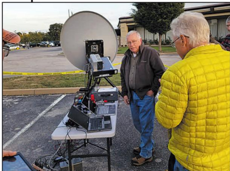
Photo B. Al Ward, W5LUA, making a 10-GHz EME (moonbounce) contact with Europe from St. Louis, Missouri at the 2016 Microwave Update conference. (Photos B-M by KOØZ)
