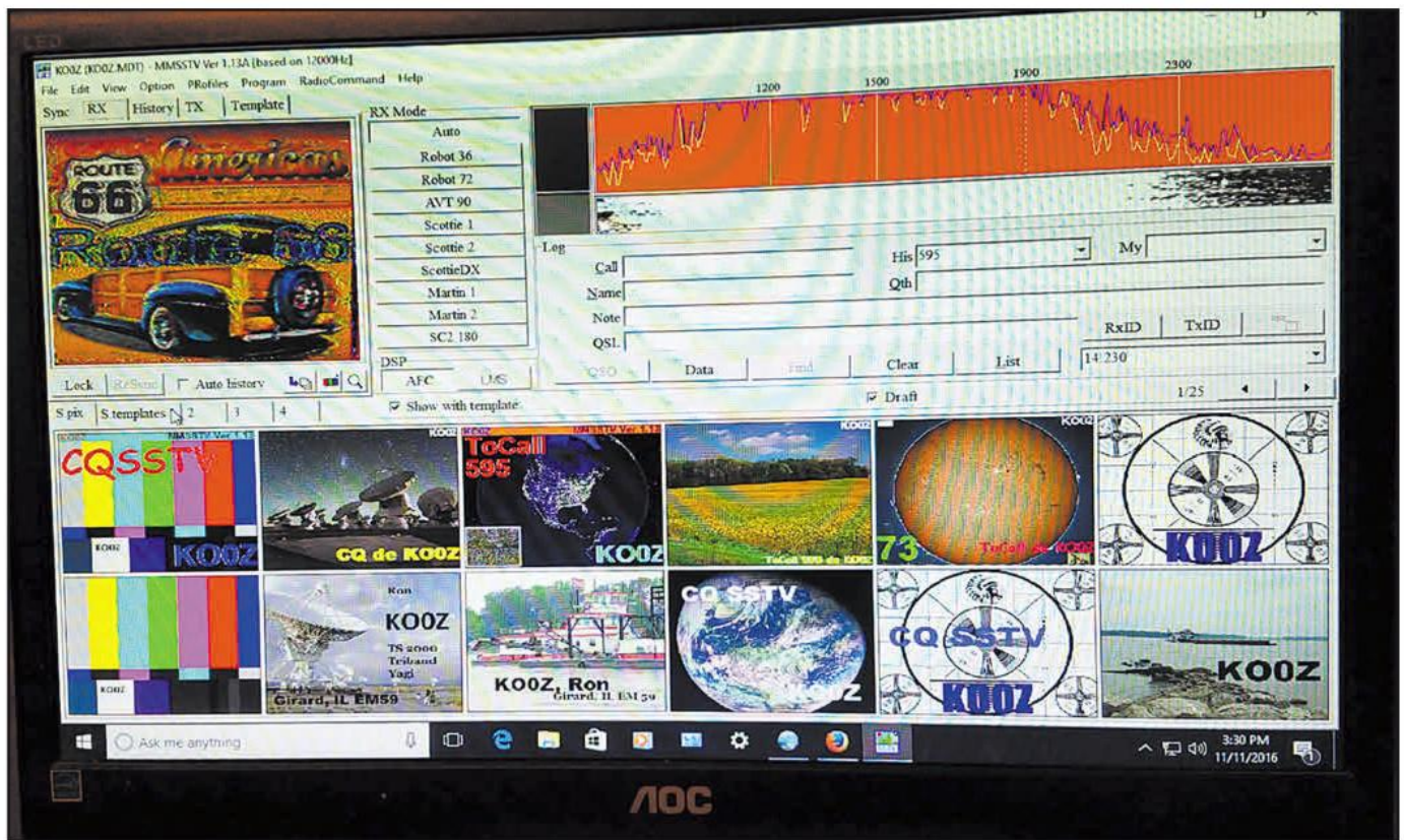
Photo H. What MMSSTV looks like on the computer screen. Note the receive window in the upper left-hand corner, the spectral display with waterfall in the upper right-hand corner. Transmit templates fill up the rest of the screen.
