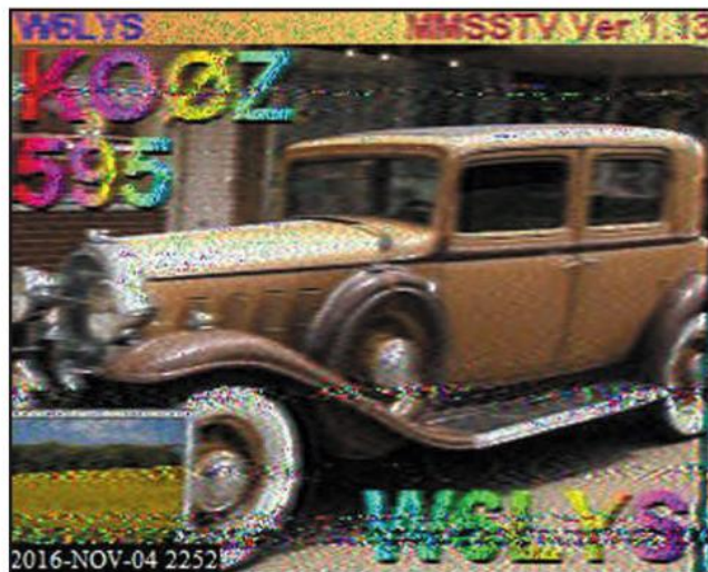
Photo D. W6LYS sending me an SSTV signal report. Note that the picture I transmitted is contained in the lower left-hand corner of Ace's return transmission.
