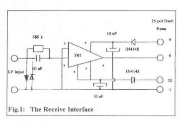
connected to a 9p Dsub and plugged into the COM port. The other end is connected across the radio's loudspeaker. The transmit interface is in principle the same
