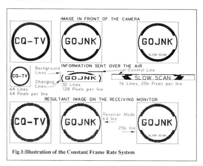
So if there is much movement then the system will be in low resolution mode with a 2 second frame rate but if you then point the camera at a still image the system will automatically switch into the highest resolution it can and send a full screen image over say 2 minutes.
