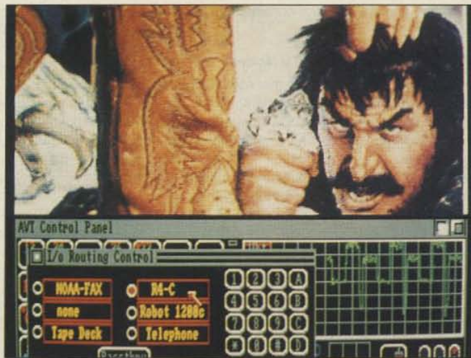
Photo C. The AVT control panel with I/O window open. The six icons on the screen are coupled to the six input jacks on the AVT interface board.
