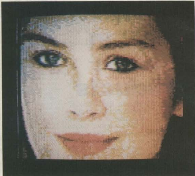
Photo G. A color-SSTV picture generated by W0LMD and placed on audio cassette tape and loaded into the TRS-80C. This picture shows the effect of color contouring. Since the display has only 256 possible colors, the shading in the flesh-tone regions are noticeable.
