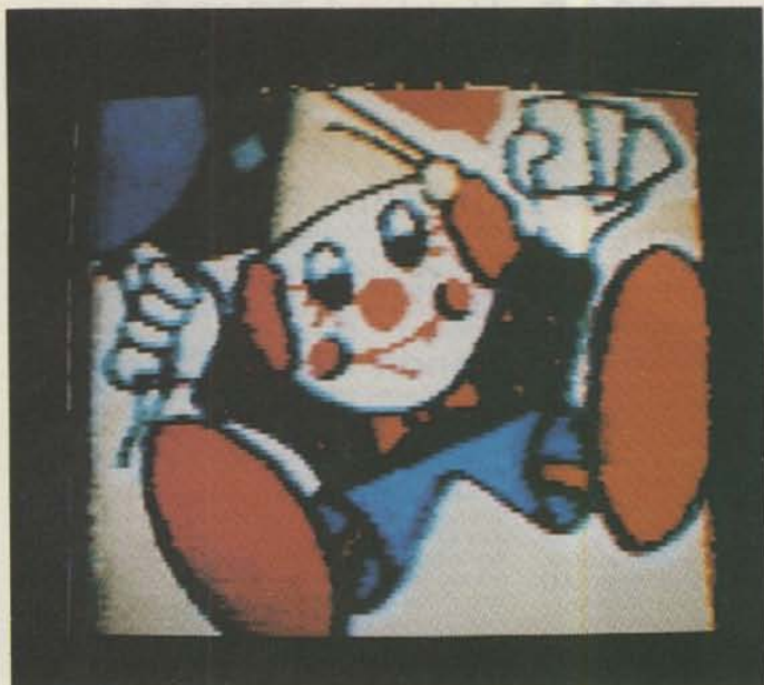
Photo F. A color-SSTV picture displayed on a TI color monitor attached to the K6AEP prototype display board. The picture was received over amateur radio on 28.680 MHz by the TRS-80C and saved on tape. The picture was generated by WB0UNB in St. Louis, Missouri.
