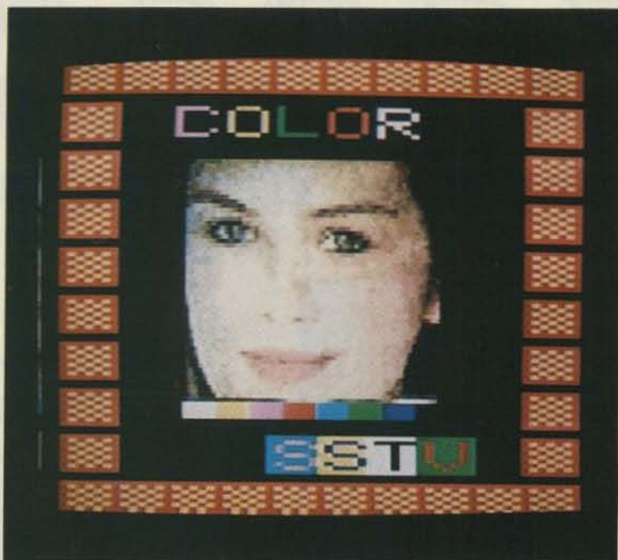
Photo H. A color-SSTV picture with graphics. This picture is the same as Photo G, but reduced in size by software and placed in the center of the image area. The graphics were generated by software and placed around the picture. The graphics and picture were all generated by the K6AEP SSTV 7.6 Revision 2 program.
