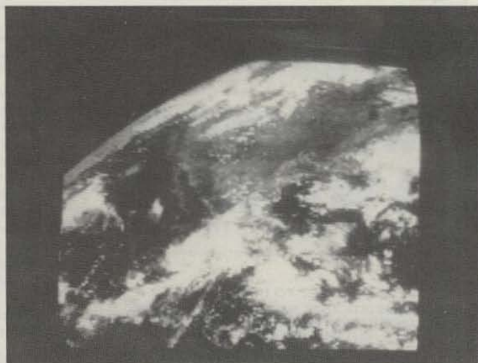
Photo B. Full-frame display of the NW quadrant of the earth as seen by GOES E in visible light. This image covers the same area as Photo A but visible-light imagery is rarely gridded. Even with the full-frame display the resolution achieved exceeds that of some small CRT display systems and is entirely adequate for most uses.
