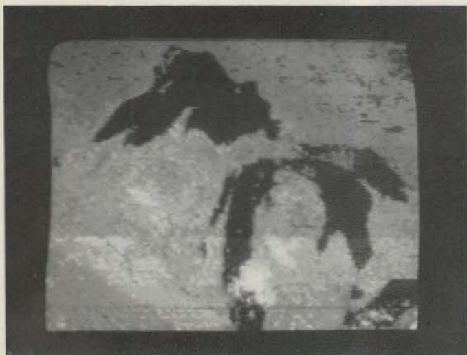
Photo G. A High Resolution 1 image obtained from a NOAA 7 visible-light APT pass showing the Great Lakes in considerable detail. A multitude of small lakes are clearly visible in southern Canada. For the ultimate in high resolution you can use the HR-2 format as shown in Photo H.
