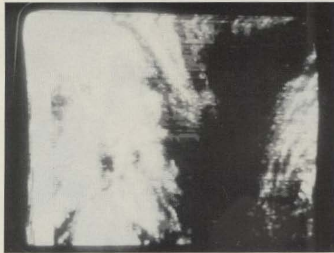
Photo J. Once the display has been optimized using the Contrast control, the image in memory can be enhanced using the contrast enhancement routine. Unlike other routines, enhancement alters the image in memory.
