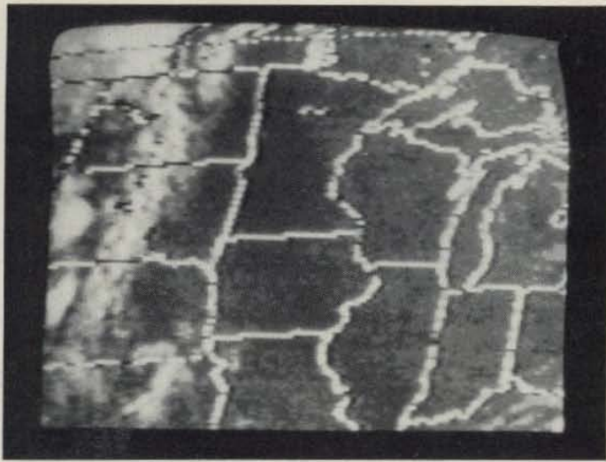
Photo E. Example of High Resolution 1 sampling of an IR WEFAX frame such as in Photo A. It shows a frontal system extending down the central Dakotas into Nebraska.
