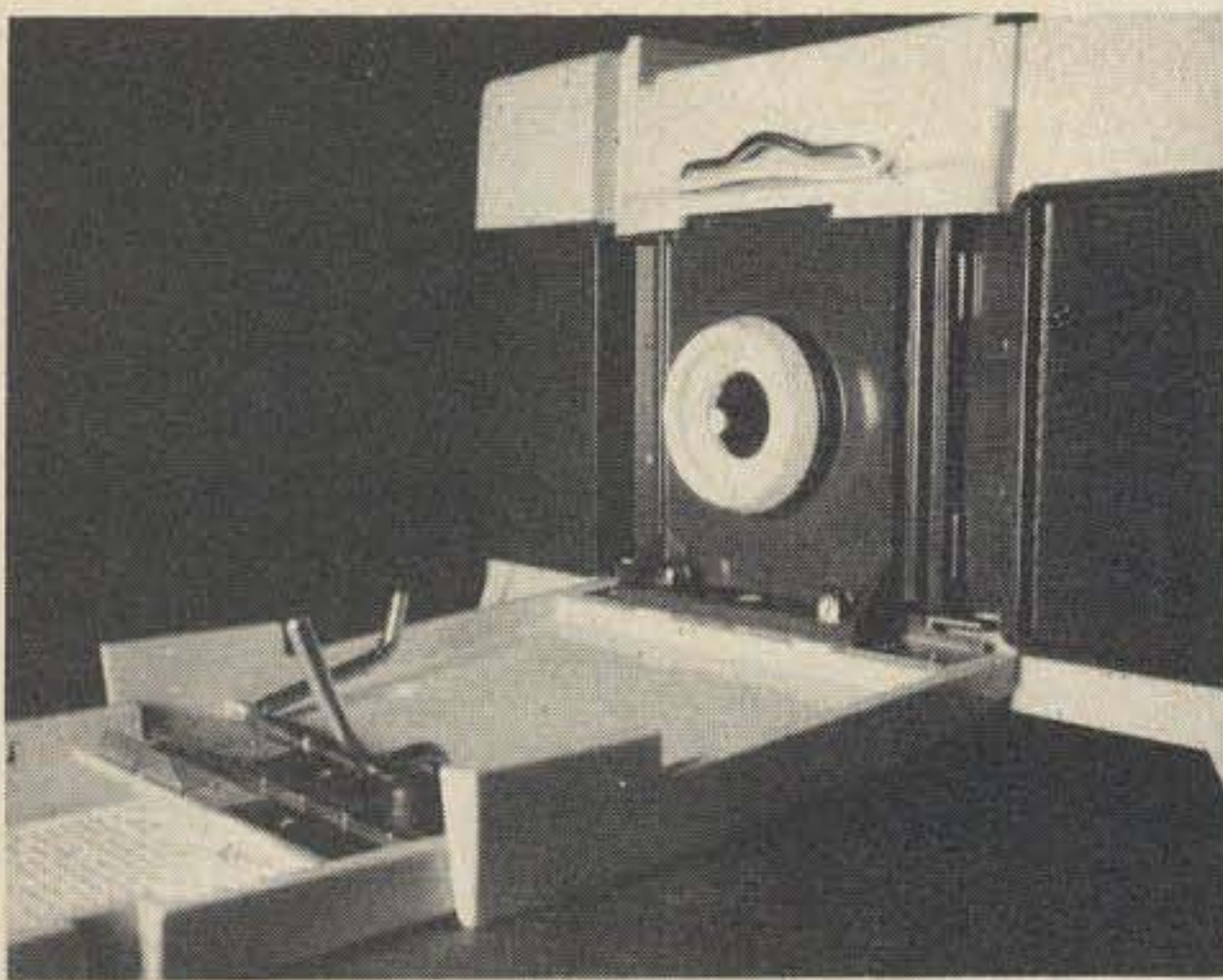
Polaroid Print Copier before modification showing the door that must be removed before copier can be used for SSTV. Notice the 2 nuts just below the lens – these are to be removed along with the pin that holds copier door to the body.
