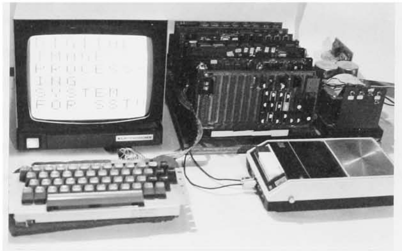
FIGURE 1B - Photograph of Digital Image Processing system for SSTV, showing the video monitor, keyboard, cassette tape recorder, and S-100 computer including the two image interface boards.
