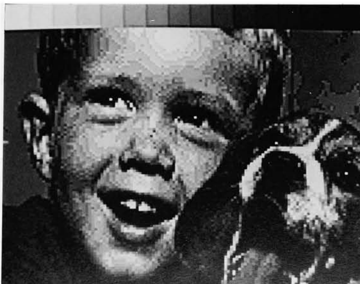
FIGURE 18B - Original Boy-Dog image after convolution with high pass kernel: 0, -1/2, 0 -1/2, 3, -1/2 0, -1/2, 0
