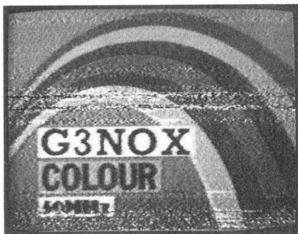
Off screen photo of G3NOX colour SSTV received in Scotland by GM3W0J via meteor scatter.
