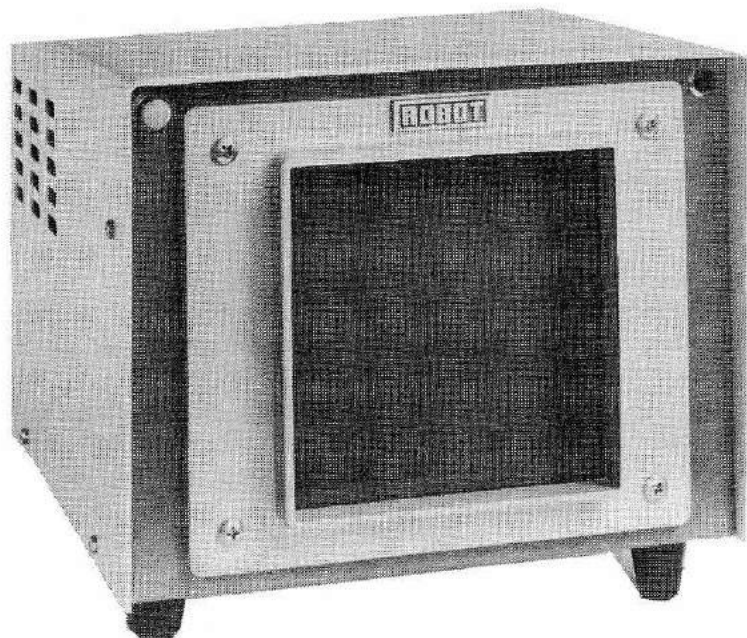
Fig. 7-6. Front view of the Robot 61 viewfinder used for display of video taken by the Robot 80 or 80A cameras.
