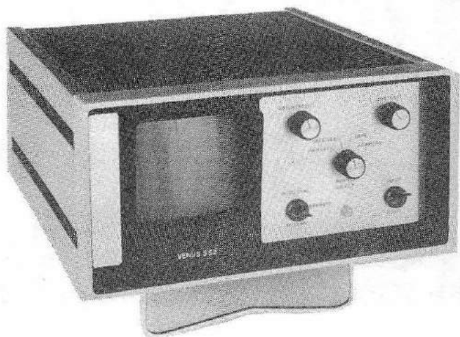
Fig. 7-12. Front view of the Venus SS2 SSTV monitor. This monitor features an Accu-Sync mode to display sync pulses on the CRT.
