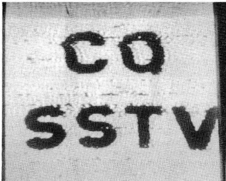
Fig. 4-2. Multipath SSTV signal. The ghost is to the right of each letter. Being very slight, this ghost indicates a low-amplitude delay signal and a strong initial signal. The salt-and-pepper effect in the picture is caused by noise.
