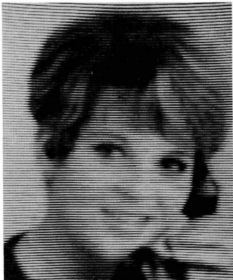
Fig. 7-3. A typical 128-line display with an 8-second time exposure from the Robot 70 monitor screen.
