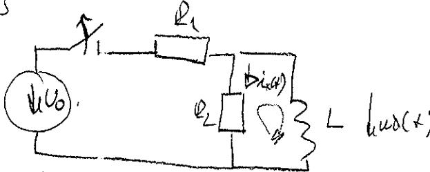
$$\begin{aligned}R_1 &= 10^3 \Omega \\R_2 &= 2.000 \Omega \\L &= 14 \\U_0 &= 10 \text{ V}\end{aligned}$$
