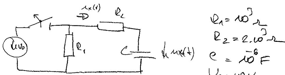
$$\begin{aligned}R_1 &= 10^3 \Omega \\R_2 &= 2 \cdot 10^3 \Omega \\C &= 10^{-6} F \\U_0 &= 10 V\end{aligned}$$
