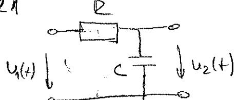
$$\begin{aligned} R &= 10^3 \Omega \\ C &= 10^{-6} F \\ U_0 &= 5V \\ U_{m1} &= 10V \\ \omega &= 10^3 \text{ s}^{-1} \end{aligned}$$
