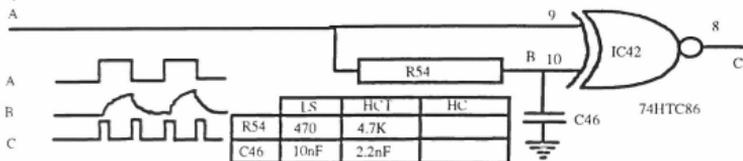
If the value of R54 and C46 are not chosen correctly then the B wave form is either too small or too high for IC42 to work and produce the C wave form. The shown approximate values have always worked so far . As a first attempt to cure the problem make sure that the value of R54 is correct and then increase the value of C46 by say 15 to 20 % . If an oscilloscope is available then adjust this time constant ( C 46 and R 54) until these wave forms are obtained.
