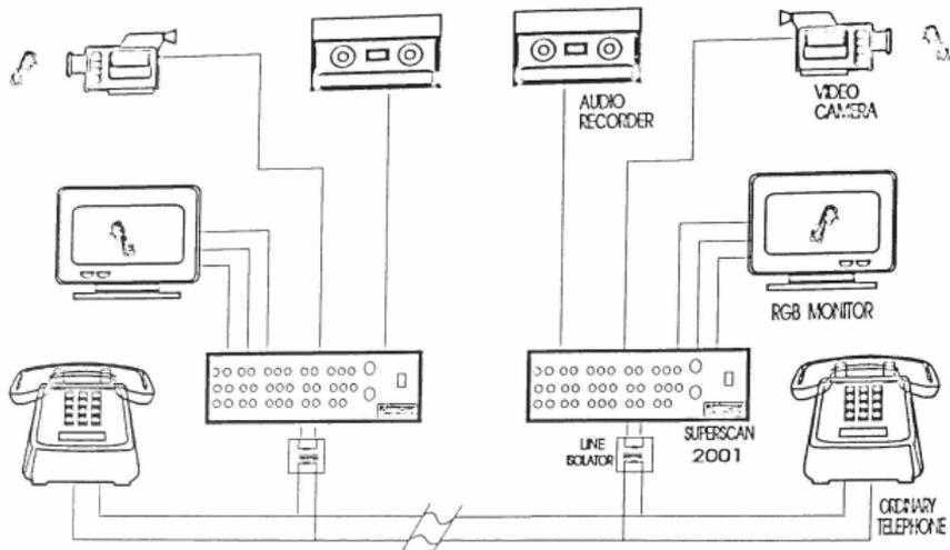
FIG. 1.1 SSTV VIA TELEPHONE LINK
